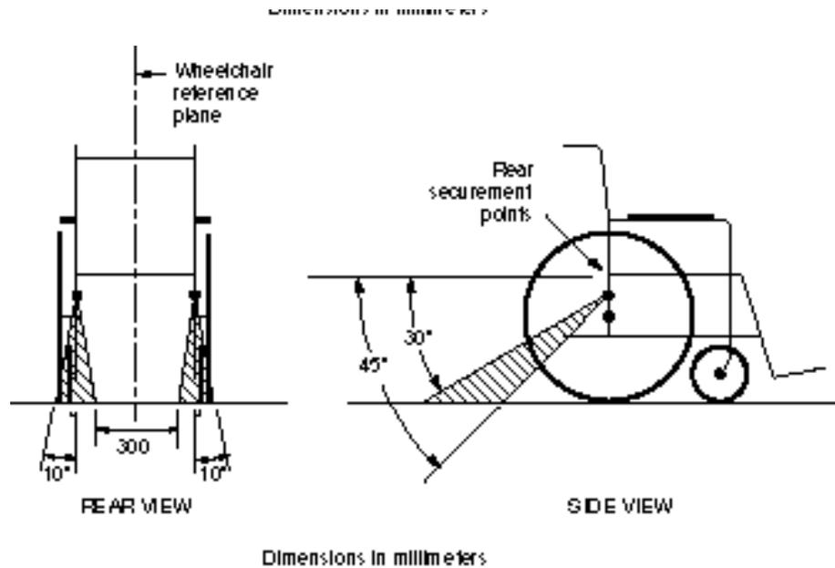
**Figure 9**-Preferred angles and locations of rear wheelchair tiedown straps and vehicle anchor points. Note that angles indicated are obtained by projecting the angle of each tiedown strap onto a vertical plane parallel to the wheelchair reference plane (side view) or onto a vertical plane that is perpendicular to the wheelchair reference plane (rear view).
