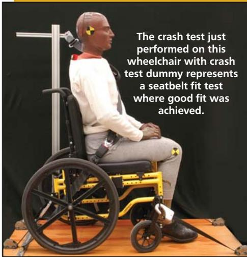
The crash test just performed on this wheelchair with crash test dummy represents a seatbelt fit test where good fit was achieved.
