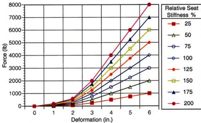
**Figure 2.** Seat stiffness scenarios evaluated in parametric analysis.
