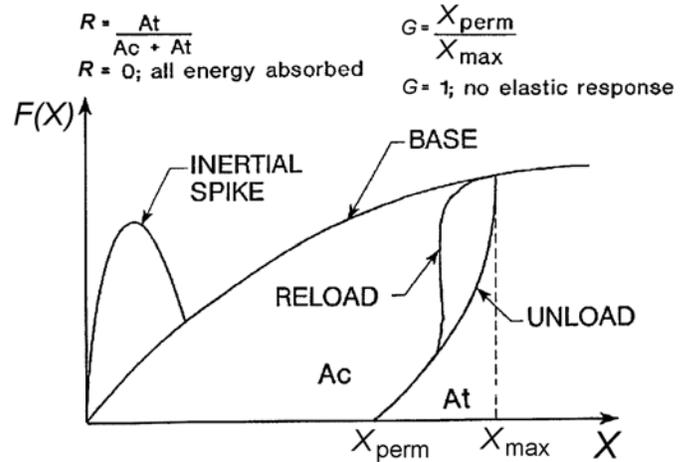
**Figure 3.** Force-deformation curve: *R* (energy absorption factor) and *G* (permanent deflection factor) equations and graphical depiction of energy absorption and energy returned; permanent deformation ( $X_{perm}$ ), maximum deformation ( $X_{max}$ ), energy absorbed ( $A_c$ ), and energy returned ( $A_t$ ).
