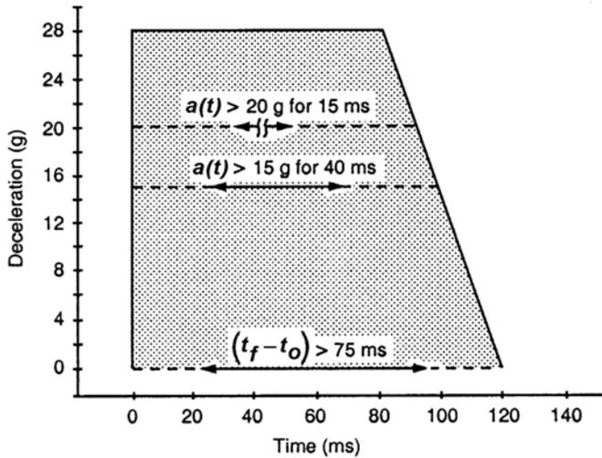
**Figure 1.** ANSI/RESNA WC-19 20 g/30 mph frontal impact deceleration pulse. Note: Acceleration and deceleration of impact sled must stay within shaded area and exceed indicated levels for specified continuous (unbroken arrows) and cumulative (broken arrows) time periods.
