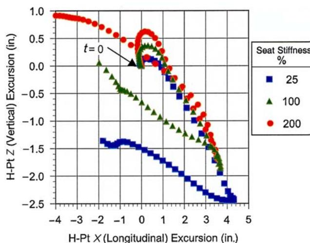
**Figure 4.** Trajectory of H-pt vertical and horizontal excursion for various seat stiffness scenarios.
