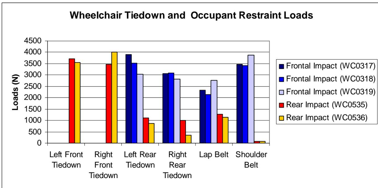
Figure 6: A comparison of wheelchair tiedown and occupant restraint loads for rear and frontal impact
