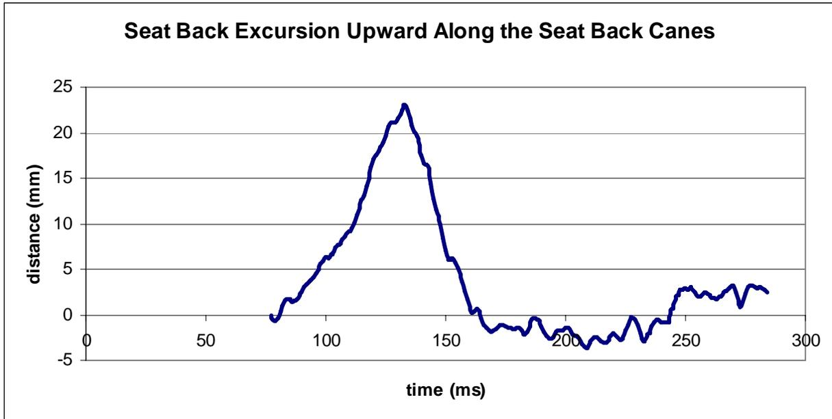
Figure 5: Seat back excursion upward along the seat back canes for rear impact test WC0536
