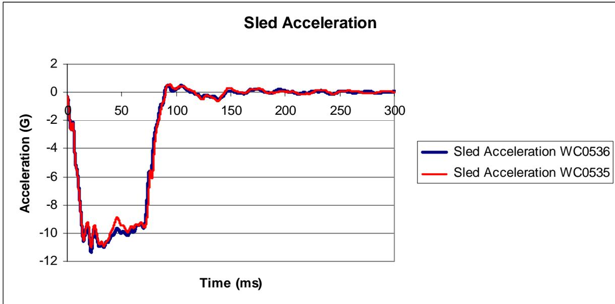
Figure 1: Sled accelerations for rear impact tests
