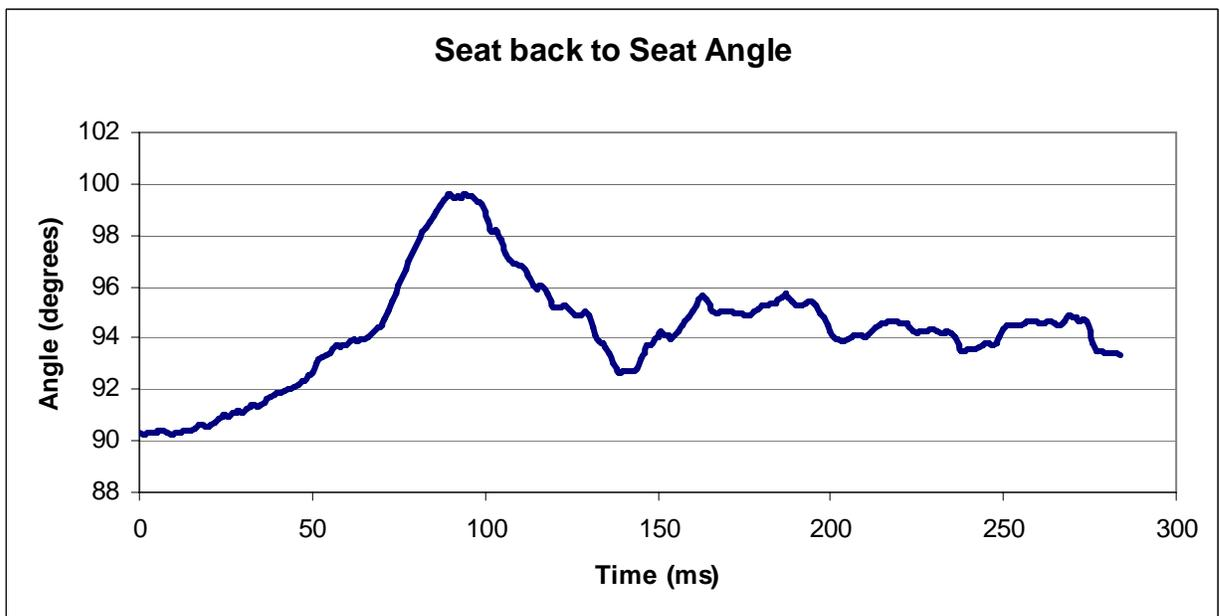
Figure 4: Seat back to seat angle for rear impact test WC0536
