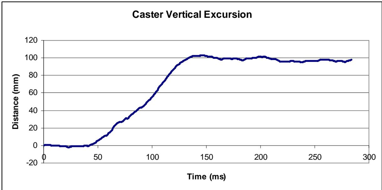
Figure 3: Caster vertical excursion for rear impact test WC0536
