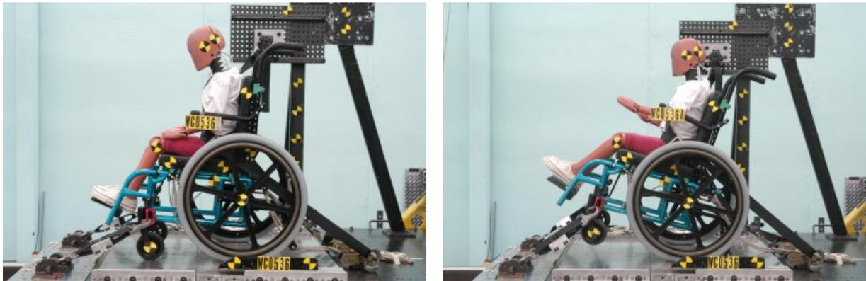
Figure 2: Photos of the experimental set up before and after the crash test.
