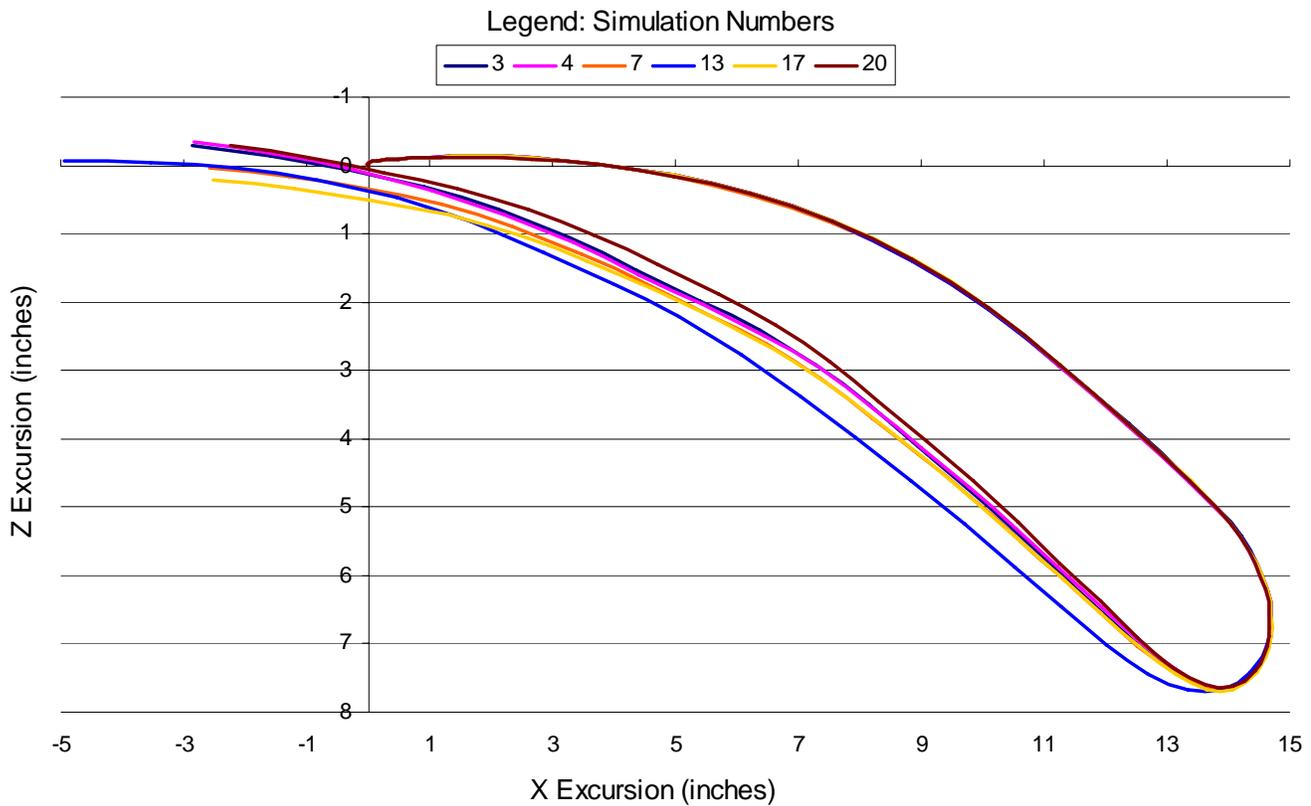
Figure 5. Head CG X-Z excursions for caster stiffness of 1750 lbs/in (original model stiffness) from time 0 to 200 msec. At x = 0 (inches) and z = 0 (inches), t = 0 (msec)
