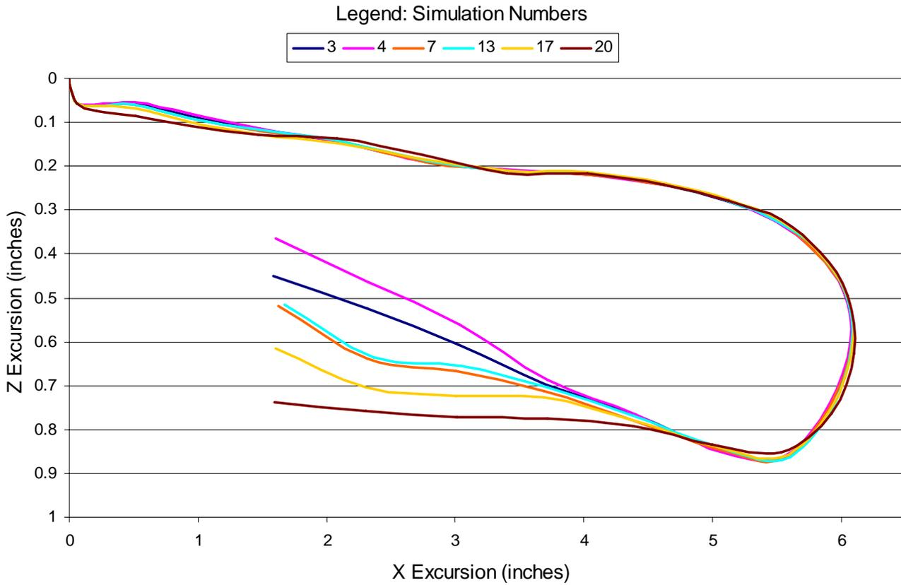
Figure 4. Wheelchair CG X-Z excursions for caster stiffness of 1750 lbs/in (original model stiffness) from time 0 to 120 msec. At  $x = 0$  (inches) and  $z = 0$  (inches),  $t = 0$  (msec)
