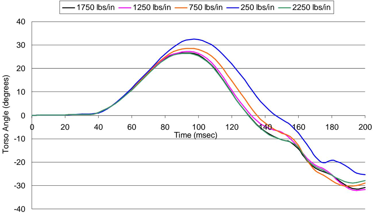
Figure 2. Torso angles relative to the vertical for various caster stiffnesses. A Positive angle indicates rearward torso rotation.
