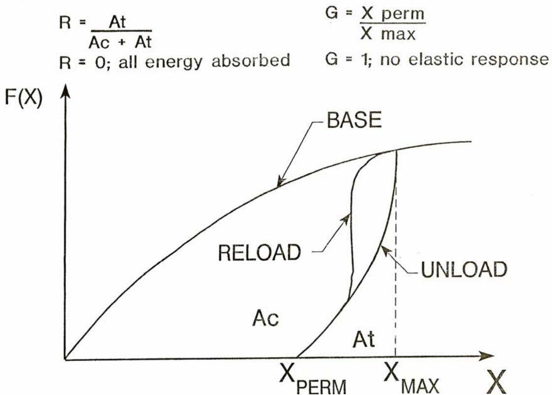
Figure1. An illustration of a force-deformation curve along with the equations for the R and G factors. Diagram depicts a loading function (BASE), an unloading function (UNLOAD), and a reloading function (RELOAD). Also the permanent deformation ( $X_{perm}$ ), maximum deformation ( $X_{max}$ ), energy absorbed ( $A_c$ ) and energy recovered ( $A_t$ ) are shown.
