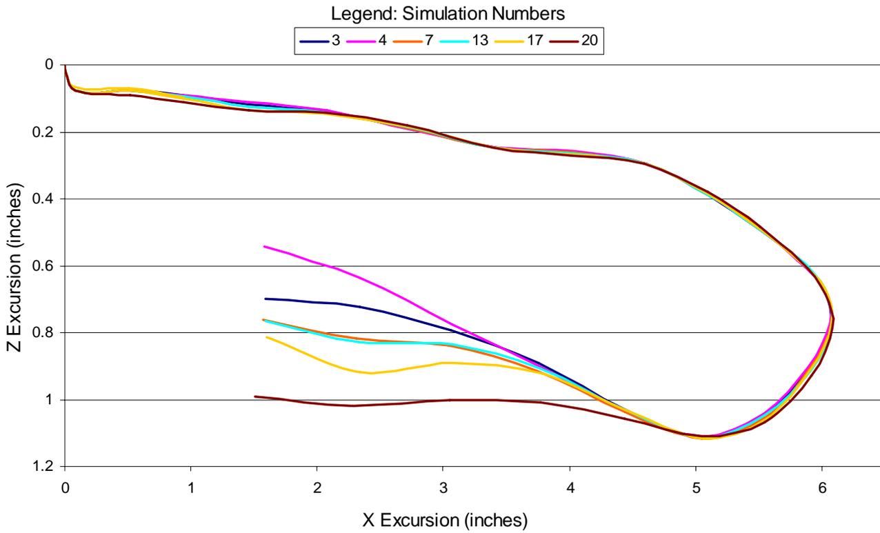
Figure 7. Wheelchair CG X-Z excursions for caster stiffness of 750 lbs/in showing from time 0 to 120 msec. At  $x = 0$  (inches) and  $z = 0$  (inches),  $t = 0$  (msec)
