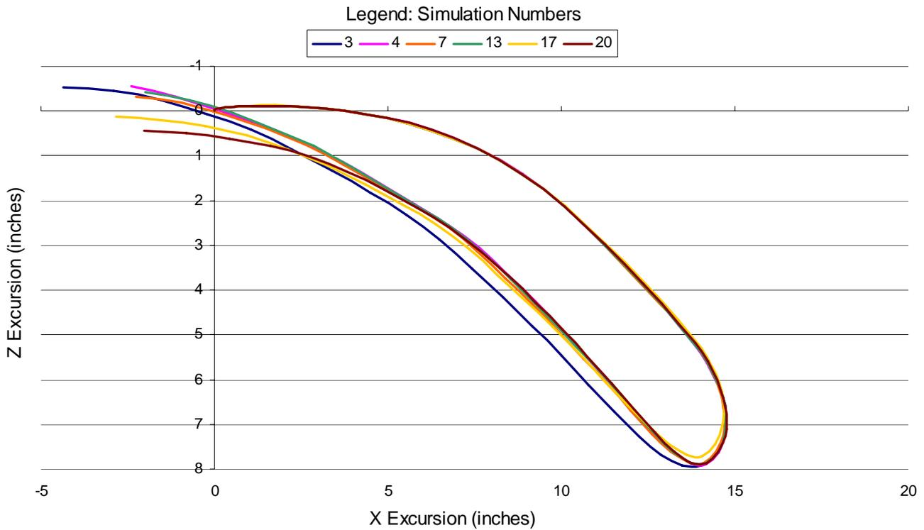
Figure 8. Head X-Z excursions for caster stiffness of 750 lbs/in from time 0 to 200 msec. At x = 0 (inches) and z = 0 (inches), t = 0 (msec)
