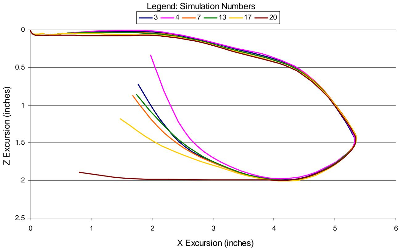
Figure 6. Caster hub X-Z excursions for caster stiffness of 750 lbs/in from time 0 to 120 msec. At  $x = 0$  (inches) and  $z = 0$  (inches),  $t = 0$  (msec)
