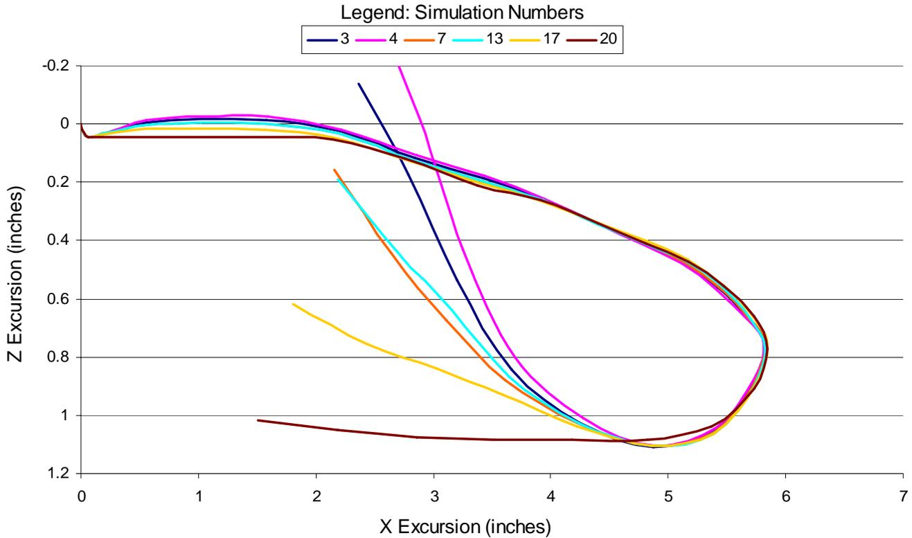
Figure 3. Caster hub X-Z excursions for caster stiffness of 1750 lbs/in (original model stiffness) from time 0 to 120 msec. At  $x = 0$  (inches) and  $z = 0$  (inches),  $t = 0$  (msec)
