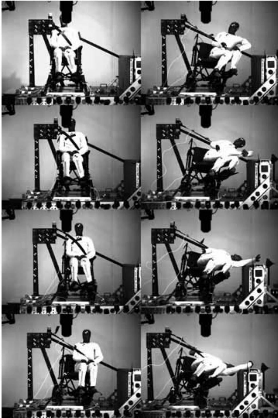
Figure 3. Sequenced images showing ATD and wheelchair motions for test A.
