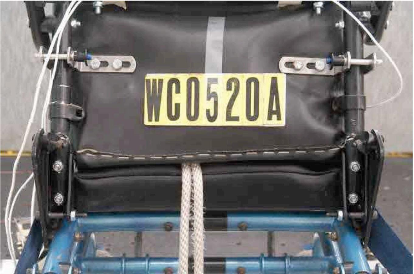
Figure 5. Rear view of seatback posts for the first prototype showing fracture of the tubing on both sides.
