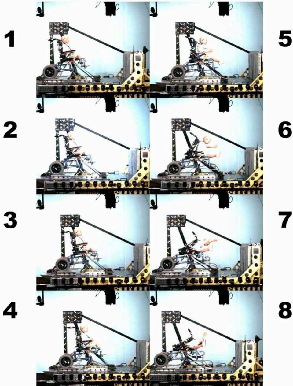
Figure 6. Time-sequence photos from test of first prototype showing high forward head excursion and head contact with lower extremities due to failure of seatback posts.
