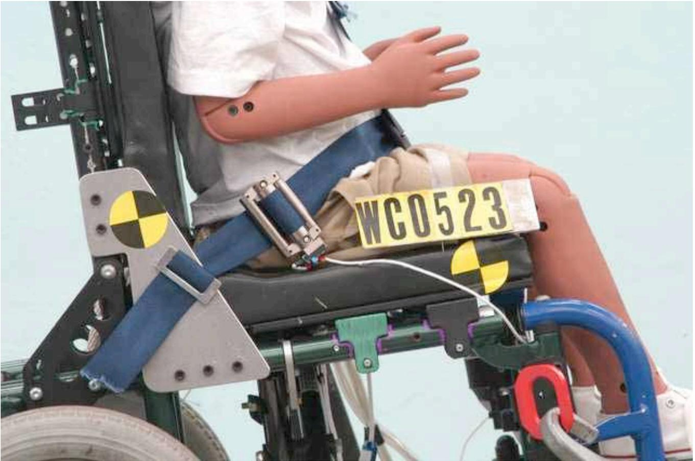
Figure 3. Side view of second prototype showing stronger bracket between seatback post and seat rail with slot for anchoring lap belt using three-bar clip.
