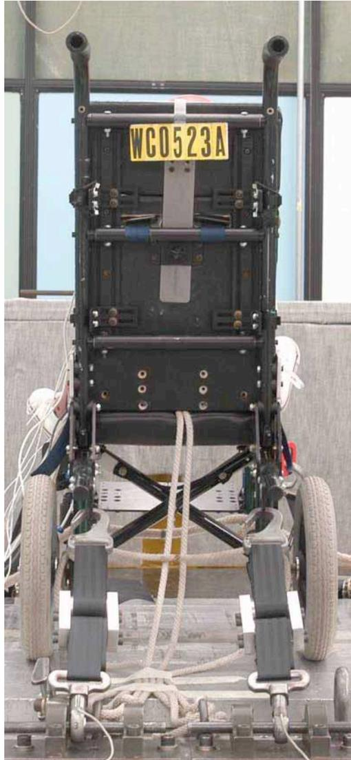
Figure 4. Rear view of second prototype showing the two transverse bars added to provide for anchoring the upper-torso belts.
