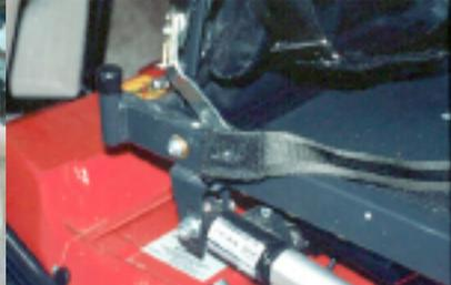
Figure 3 - Postural lap belt torn at attachment to wheelchair.
