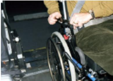
Figure 5 – View of three-point belt showing location of end-release button on receptacle.
