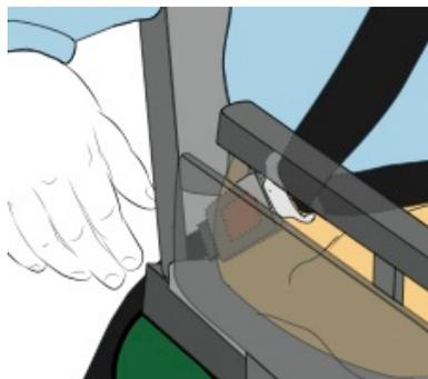
Lap belt threaded into opening between the wheelchair seat
