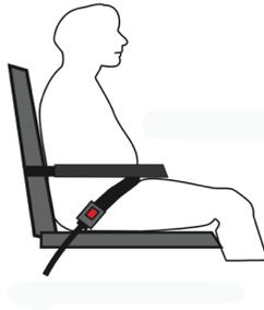
Proper positioning of a vehicle-anchored lap belt with wheelchair arm supports that are attached to the back-support posts and completely open at the front and underneath
